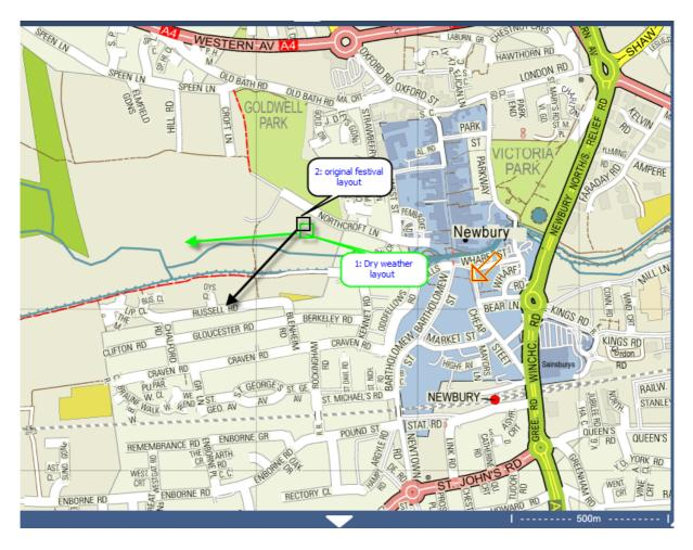
Layout / Orientation 1: This provides the most effective sound dispersion, broadcasting into open space and using the trees and the Northcroft Leisure Centre building to absorb sound.
